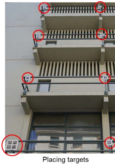
Figure 5. Experimental setup for AprilTag detection
